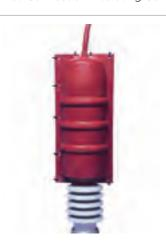
BCIC covers are designed to protect energized conductors or busbars from flashovers due to contact from birds, squirrels and other wildlife. BCIC parts are made from a UV stable, track resistant, high performance TE Connectivity material to ensure years of reliable service.
