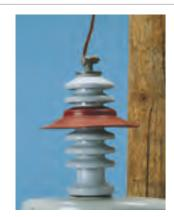
Heat-shrinkable creepage extenders help to increase the flashover performance of insulators by reducing the surface electrical stress and leakage current and increasing the creepage length of the insulators. The extenders are designed to be resistant to conventional spray washing techniques and will withstand most normal handling, abuse, and extreme weather conditions.
