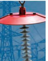
The rigid red guano shield protects against bird streamer caused outages. There are designs to fit both porcelain bells and polymeric insulators. This two piece shield attaches easily with plastic bolts and nuts around the top of the insulator and provides protection from fecal contaminates coming from above the insulator string. For both applications there are 450 mm and 600 mm diameter shield
