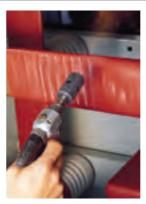
HVBT tape is an adhesive coated, high-voltage, heat-shrinkable, general-purpose tape for insulating straight and bent bars in retrofit applications where tubing cannot be used. In addition, HVBT easily insulates unusual connections and geometries in the factory or field.
