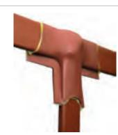
HVIS is an adhesive coated, heat-shrinkable sheet that shrinks in two directions to tightly conform to complex shapes. It is ideal for insulating busbar tees, elbows, and other connections where tubing or tape cannot be used. HVIS may also be used in conjunction with Raysulate electrical insulating tapes and tubings or alone to help protect against accidental bridging caused by birds and animals.
