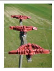
The Birdcap family of insulating covers are specifically designed to protect birds from causing flashovers during take-off, landing and perching on energised conductors at crossarm and poletop insulators. This also protects the network from outages and potential damage to equipment and conductors.
