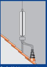
Roof cable/pipe entry system for ridged roofs Example installation: Connection of a mobile communications antenna
