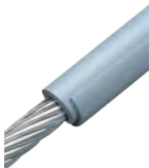
Medium Voltage Conductor Covers (MVCC) provide high quality electrical insulation for substation leads and jumpers. These covers are made from a non-tracking silicone material that is suitable for harsh medium voltage outdoor environments. MVCC covers are split for easy installation.
