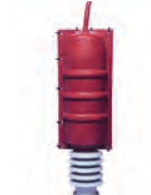
BCIC covers are designed to protect energized conductors or busbars from flashovers due to contact from birds, squirrels and other wildlife. BCIC parts are made from a UV stable, track resistant, high performance TE Connectivity material to ensure years of reliable service.
