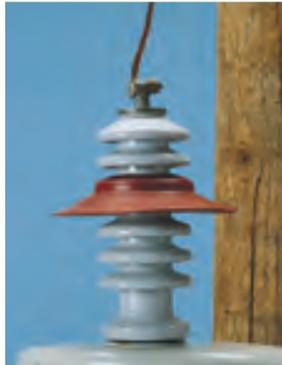
Heat-shrinkable creepage extenders help to increase the flashover performance of insulators by reducing the surface electrical stress and leakage current and increasing the creepage length of the insulators. The extenders are designed to be resistant to conventional spray washing techniques and will withstand most normal handling, abuse, and extreme weather conditions.
