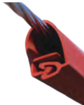
The MVLC cover is a cold-applied wrap-around cover that provides retrofit insulation for overhead conductors to help prevent electrical outages caused by incidental contact from tree branches or wildlife.
