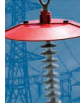
The rigid red guano shield protects against bird streamer caused outages. There are designs to fit both porcelain bells and polymeric insulators. This two piece shield attaches easily with plastic bolts and nuts around the top of the insulator and provides protection from fecal contaminates coming from above the insulator string. For both applications there are 450 mm and 600 mm diameter shield designs.
