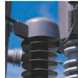
These insulating covers are designed to prevent bird caused outages on distribution equipment ranging from 15 to 36 kV. Covers are available for terminations, reclosures, lightning arresters, and fuse cutouts.
