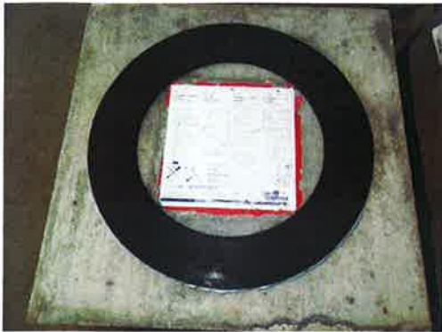
Figure 3. Test specimen before the installation of the clamping bell.
