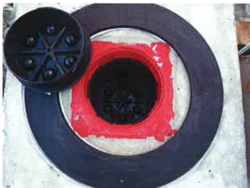
Figure 8. Test specimen after removal of the compression bell and sealing cap.
