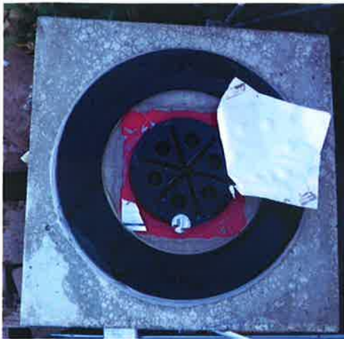
Figure 7. Test specimen after removal of the compression bell and protective foil.
